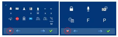
3. Pressing  $\checkmark$ , select the desired access 4. Press \*, to exit to the previous menu. mode, in the selected option. Activation is confirmed since the white line stops blinking and remains constant.
