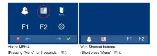
**Note:** When communicating or only with video, pressing the Menu button twice displays the shortcut buttons.
