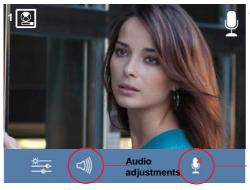
**1.** Select the audio adjustments option with the corresponding capacitive button.
