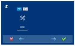
Select the default parameters option via the cursors (white line under the icon) and press ✓. The monitor exits the menu and starts to save the selected option. This status is displayed, since it sequentially goes through all capacitive buttons, indicating that the reset is being performed.
