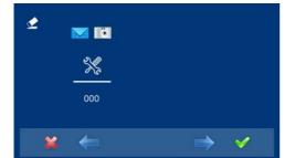
Select the default parameters option via the cursors (white line under the icon) and press ✓. The monitor exits the menu and starts to save the selected option. This status is displayed, since it sequentially goes through all capacitive buttons, indicating that the reset is being performed.
