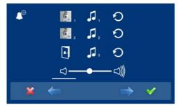
Select the audio adjustments option via the cursors(white line under the icon) and press ✓. While in audio adjustments, use the capacitive buttons to obtain the desired settings.
