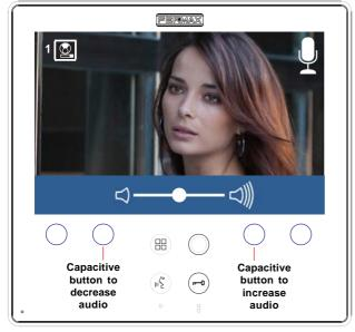
While in audio adjustments, use the capacitive buttons to obtain the desired settings.
