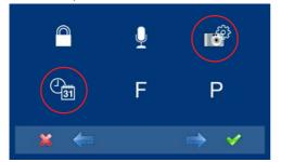
receiving the call. With this option selected with the cursors (white line under the cursor), press ✓, if you want to remove the selection, you also press ✓. Press ×, to exit to the previous menu and confirm the selected options. Continue pressing × until you reach the desired menu or you exit programming.
