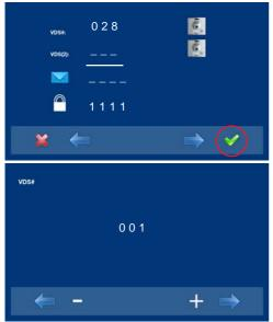
1. Select the programming option from the monitor VDS (2). The selected option is displayed with the white line under the icon.
